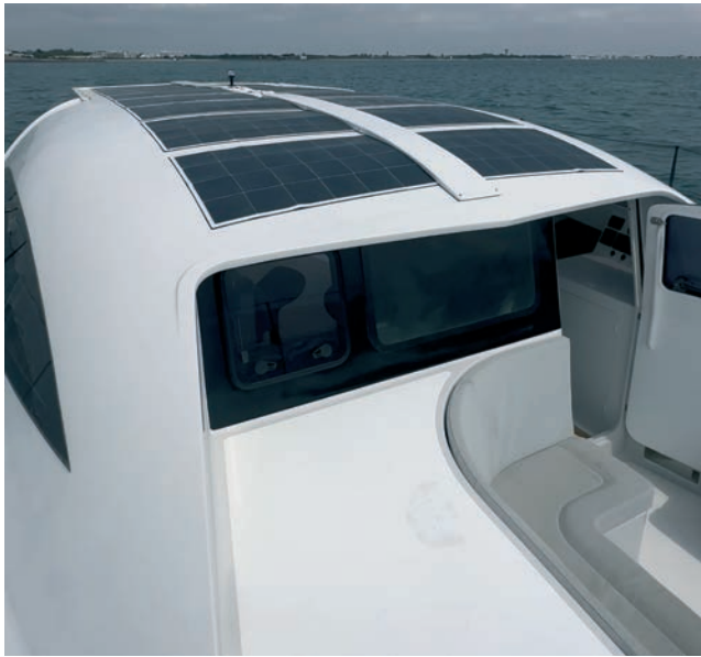
On the current version, the coachroof is equipped with 2 kWp of solar panels, but upcoming modifications will double this charging capacity.
