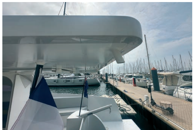
At the after end of the roof, two small pipes channel rainwater directly into the tanks.
