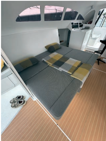
Like the legs of the convertible table in the saloon, carbon fiber elements highlight the importance of weight reduction on an electrically powered boat.
