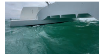
The long sugarscoops, great for swimming or getting in the dinghy, are also very practical alongside for stepping aboard, even from the side thanks to the cut-out sections. The bridgedeck clearance is high enough to allow easy passage through the water.
