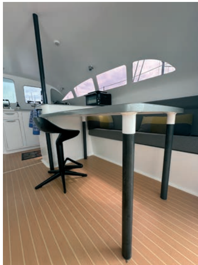
Like the legs of the convertible table in the saloon, carbon fiber elements highlight the importance of weight reduction on an electrically powered boat.
