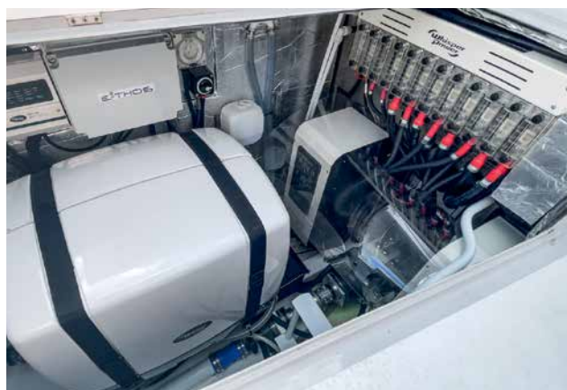
BELOW Whisperpower Genverters (in white sound-proofed boxes) kick in when needed. The electric motor can be seen at the head of the propshaft.
